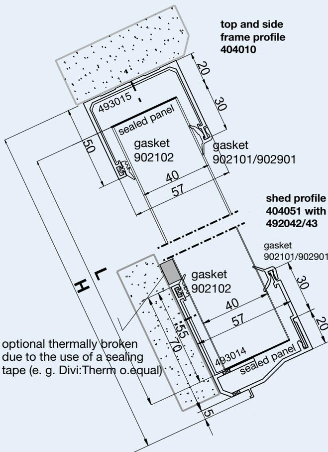
Calculation of panel length:  $L$  in mm = Height  $H$  in mm - 45 mm
