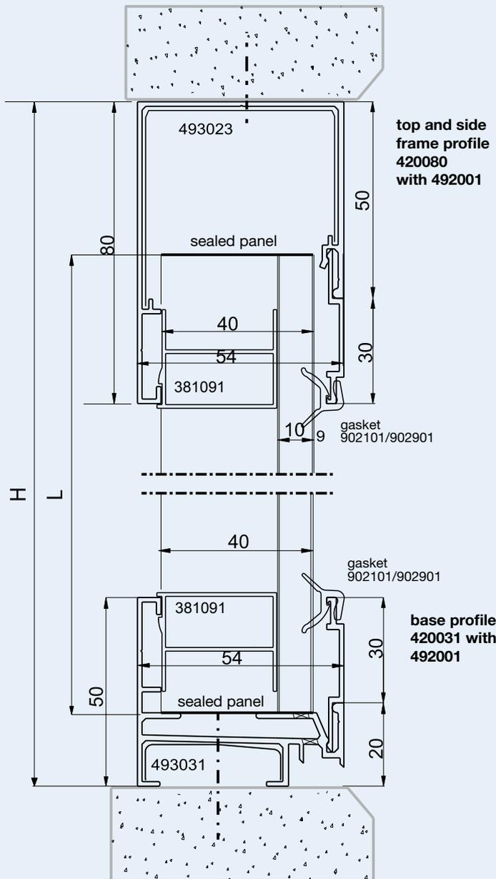
Calculation of panel length:  $L$  in mm = Height  $H$  in mm - 60 mm
