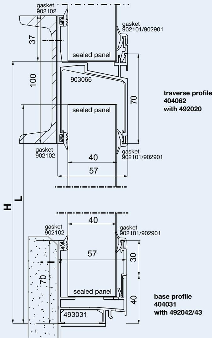
Calculation of panel length:  $L$  in mm = Height  $H$  in mm
