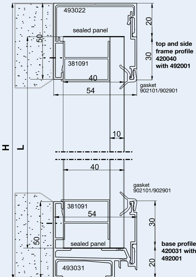
Calculation of panel length:  $L$  in mm = Height  $H$  in mm - 40 mm
