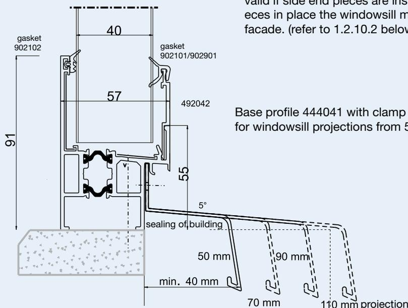
Base profile 444041 with clamp batten 492042 for windowsill projections from 50 to 110 mm
