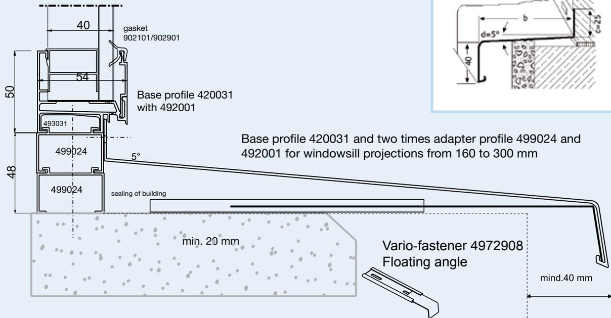
Aluminium windowsills should project approx. 40mm over the ready facade. Accordingly the profile width needs to be measured. This is only valid if the side end pieces are installed as well. Without side end pieces the windowsill must project 20mm over the ready facade (refer to 1.2.10.2).
