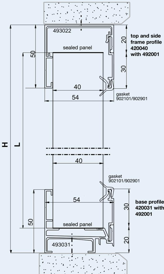
Calculation of panel length:  $L$  in mm = Height  $H_0$  in mm - 40 mm
