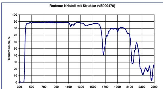
The measurement of the transmission values was carried out with application of a natural day light lamp of 20,000 Lux in connection with a lux meter Lightmeter MS 1000-300 – measuring range 200 to 50,000 LUX) exemplarily on a 1 mm thick PC.
