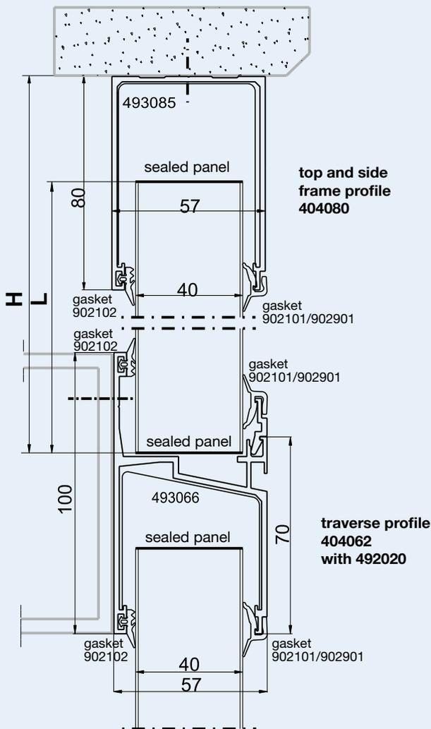
Calculation of panel length:  $L$  in mm = Height  $H$  in mm - 45 mm
