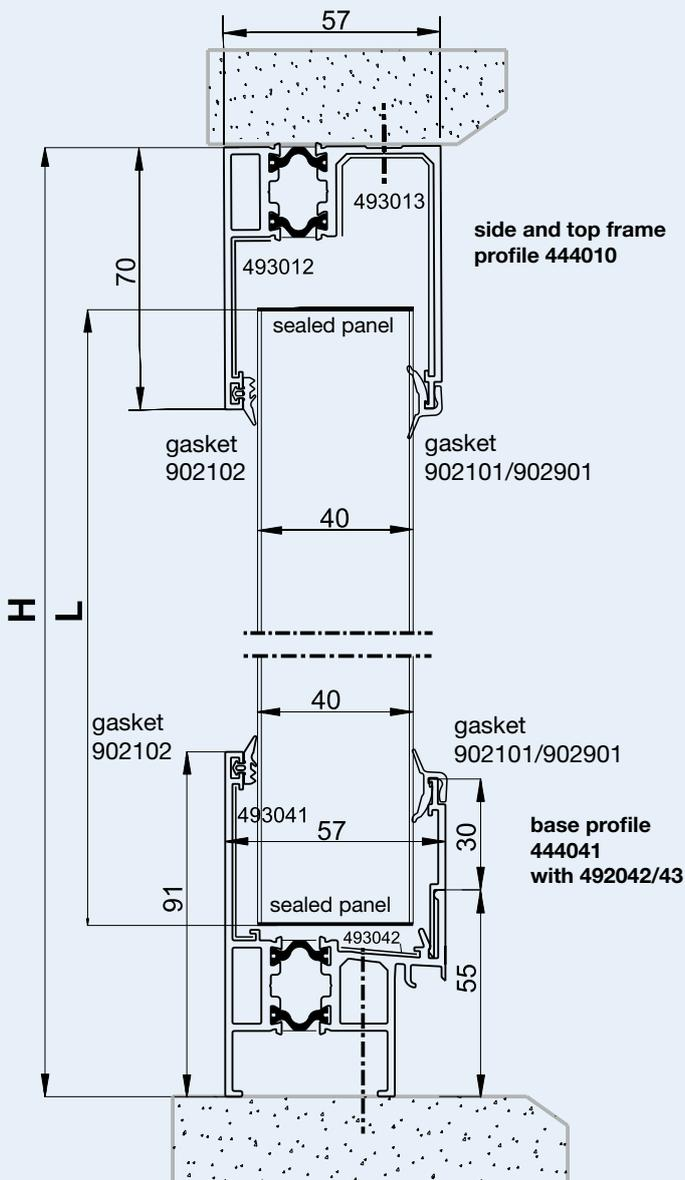
Calculation of panel length:  $L \text{ in mm} = \text{Height } H \text{ in mm} - 90 \text{ m}$
