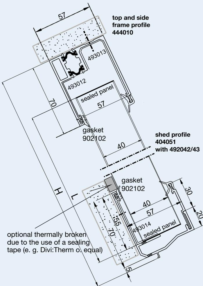
Calculation of panel length:  $L$  in mm = Height  $H$  in mm - 55 mm
