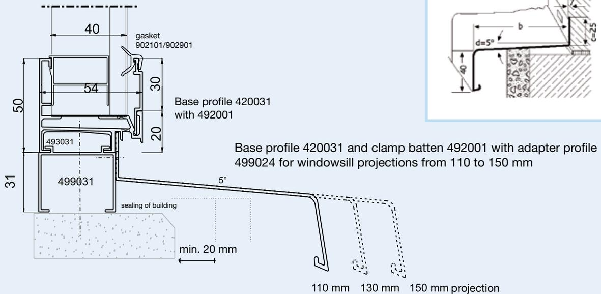
Aluminium windowsills should project approx. 40 mm over the ready facade. Accordingly the profile width needs to be measured. This is only valid if side end pieces are installed as well. Without side end pieces in place the windowsill must project 20mm over the ready facade. (refer to 1.2.10.2)
