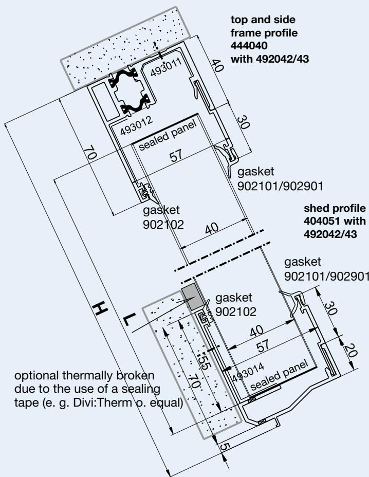
optional thermally broken due to the use of a sealing tape (e. g. Divi:Therm o. equal)
