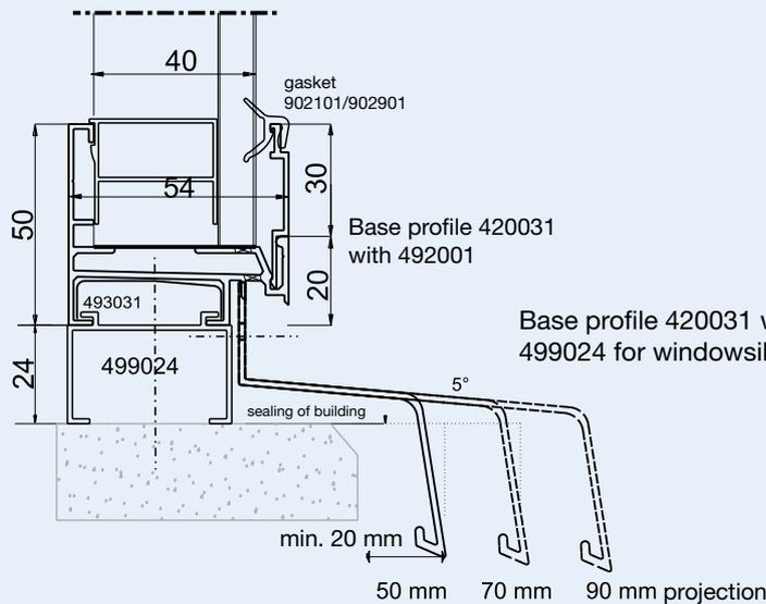
Base profile 420031 with clamp batten 492001 and adapter profile 499024 for windowsill projections from 50 to 90 mm
