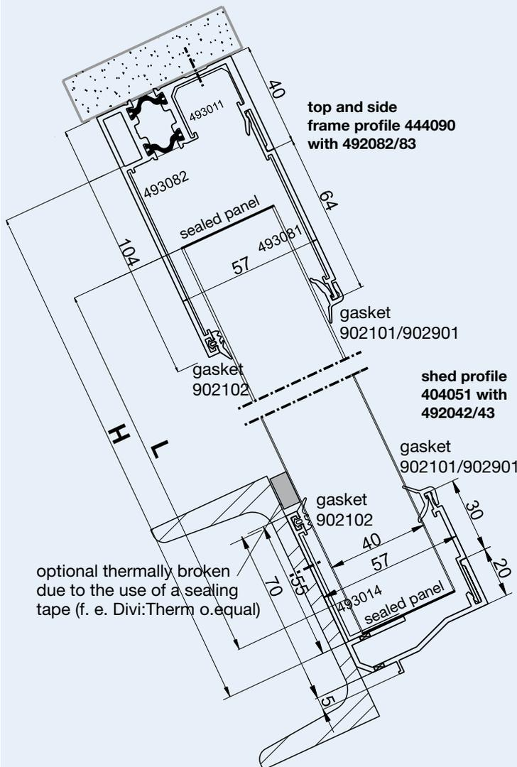
Calculation of panel length:  $L$  in mm = Height  $H$  in mm - 75 mm
