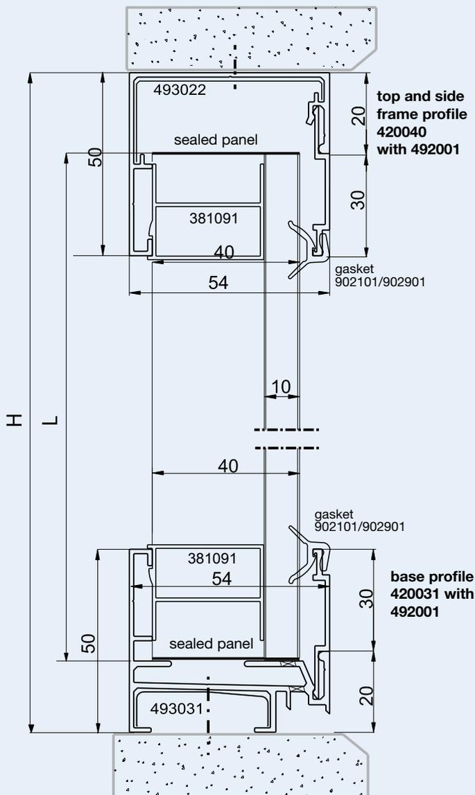
Calculation of panel length:  $L$  in mm = Height  $H$  - 40 mm
