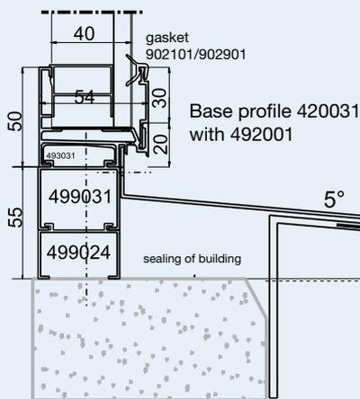
Base profile 420031 and adapter profile 499024 and 492001 for windowsill projections from 320 to 360 mm
