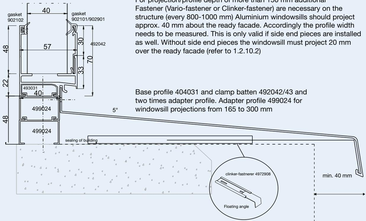
For projection/profile depth of more than 150 mm additional Fastener (Vario-fastener or Clinker-fastener) are necessary on the structure (every 800-1000 mm) Aluminium windowsills should project approx. 40 mm about the ready facade. Accordingly the profile width needs to be measured. This is only valid if side end pieces are installed as well. Without side end pieces the windowsill must project 20 mm over the ready facade (refer to 1.2.10.2)
