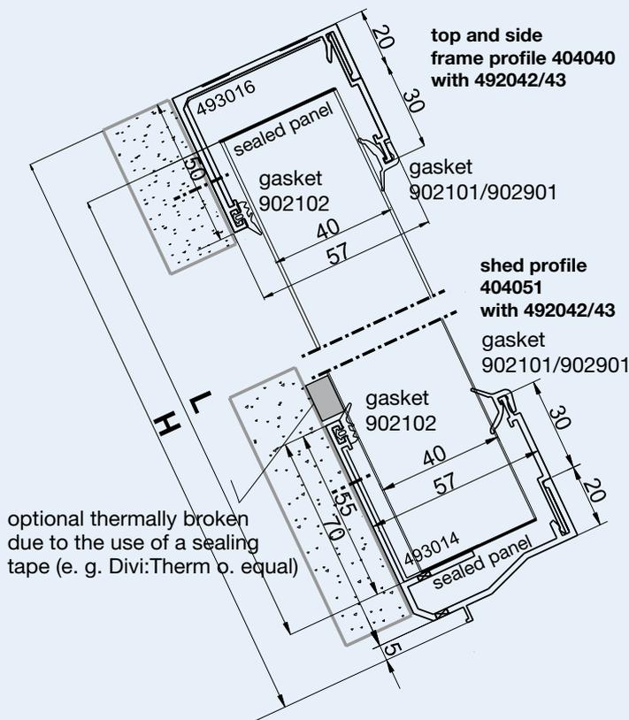
Calculation of panel length:  $L$  in mm = Height  $H$  in mm - 45 mm
