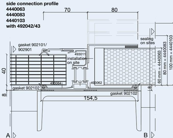
Distance of substructure to PC panel 8mm
