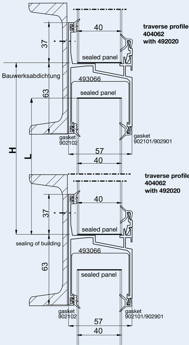
Calculation of panel length:  $L$  in mm = Height  $H$  in mm - 30 mm
