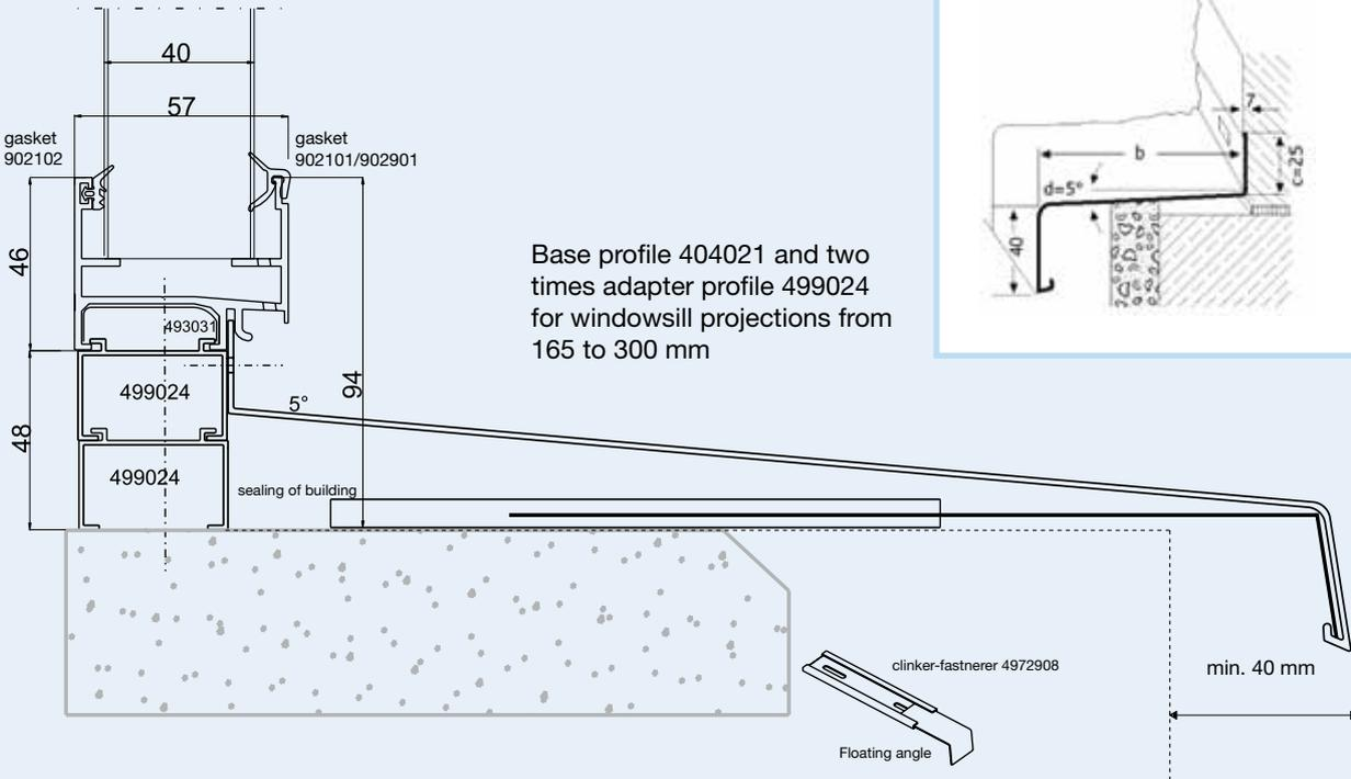
Base profile 404021 and two times adapter profile 499024 for windowsill projections from 165 to 300 mm
