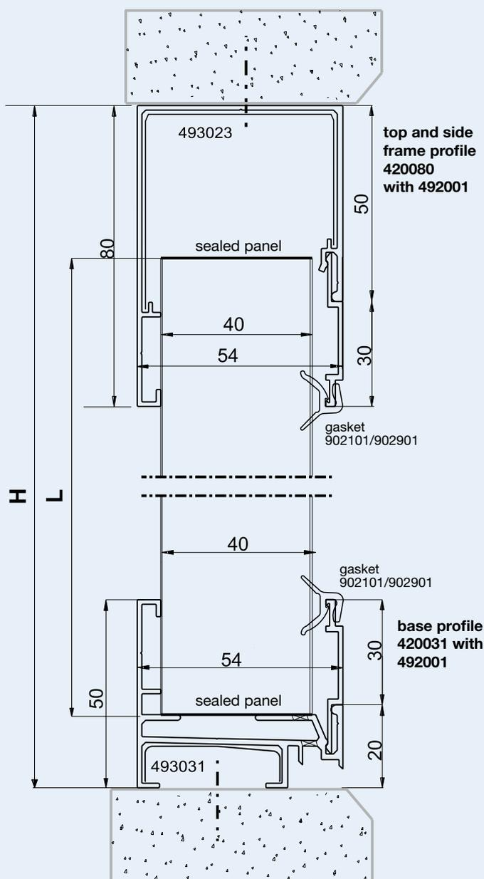
Calculation of panel length:  $L$  in mm = Height  $H$  in mm - 60 mm
