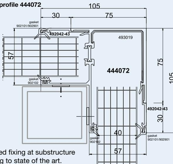
Both sided fixing at substructure according to state of the art.
