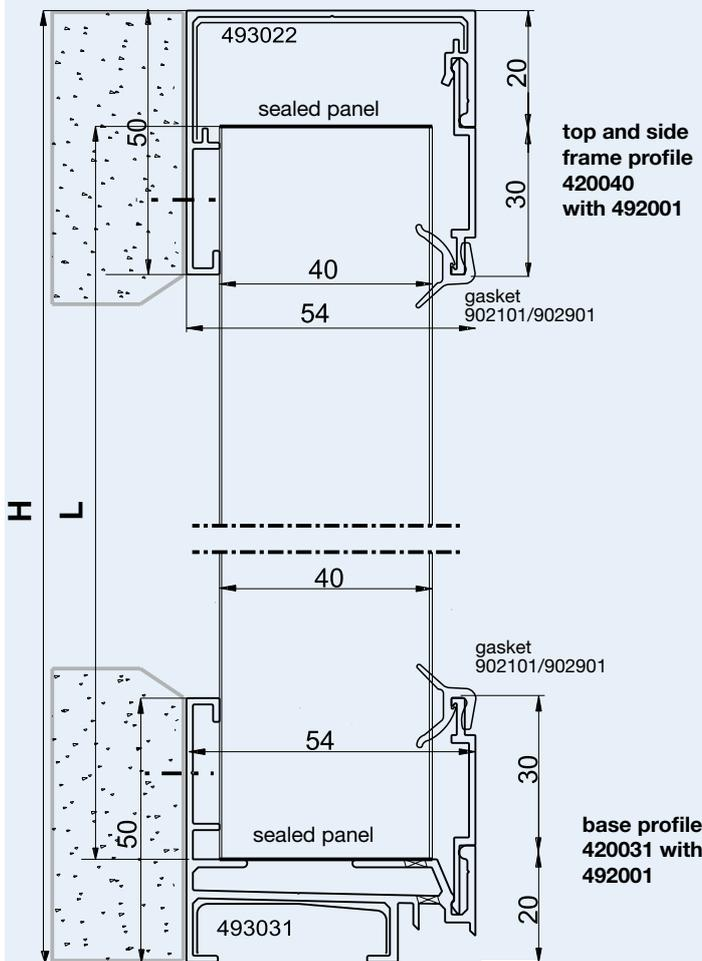
Calculation of panel length:  $L$  in mm = Height  $H$  in mm - 40 mm
