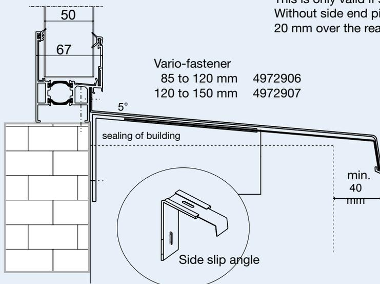
With a projection/profile depth of more than 150 mm additional fasteners (Vario-fastener or Clinker-fastener) on the structure are necessary. (every 800 to 1,000 mm)
