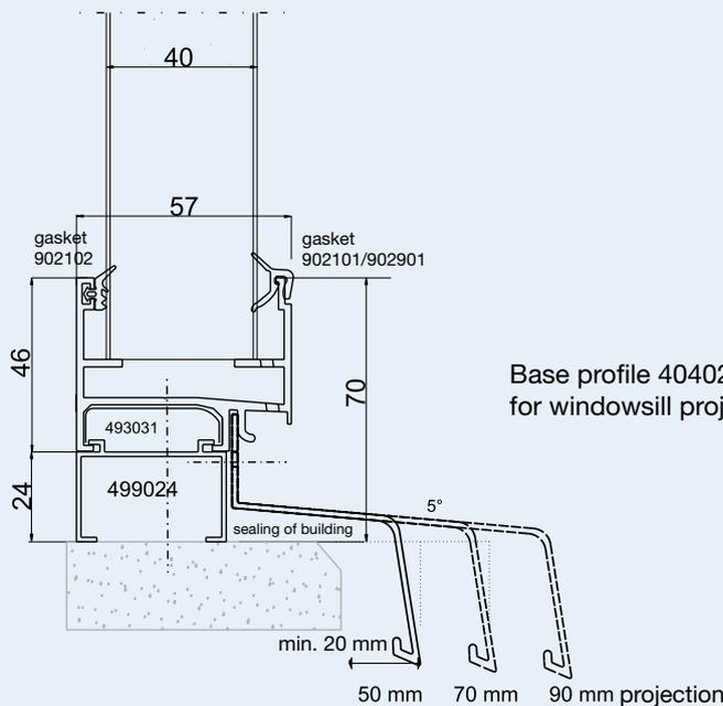
Base profile 404021 and adapter profile 499024 for windowsill projections from 50 to 90 mm
