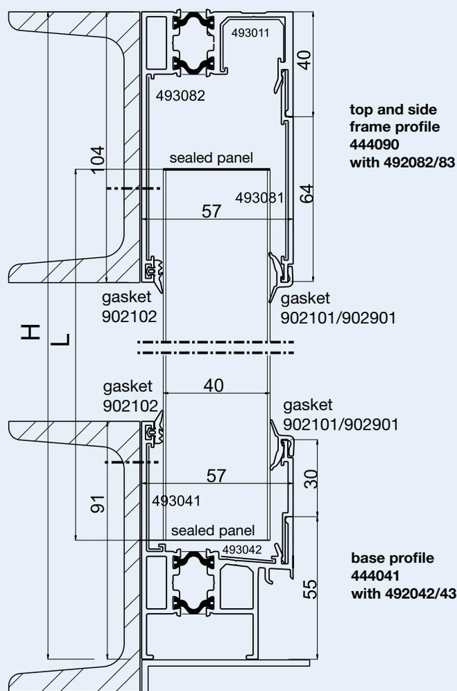
We recommend to support the base profile for panel length starting from 7.00 m
