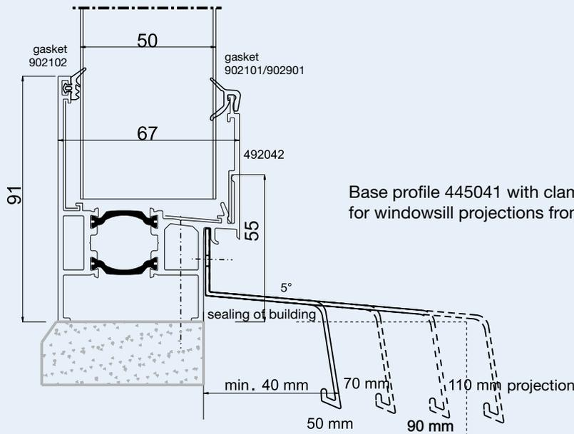
Base profile 445041 with clamp batten 492042 for windowsill projections from 50 to 110 mm
