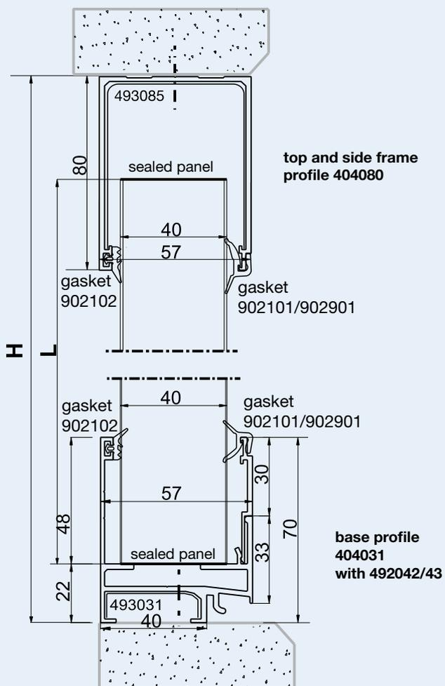
Calculation of panel length:  $L$  in mm = Height  $H$  in mm - 60 mm
