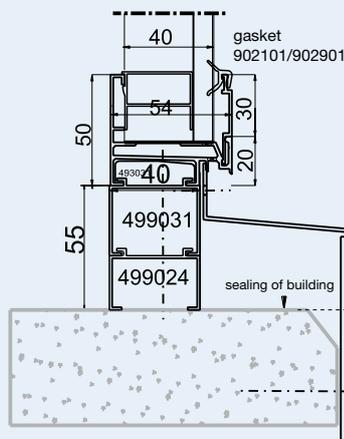
Base profile 420031 and clamp batten 492001 and adapter profile 499024/31 for windowsill projections from 320 to 360 mm
